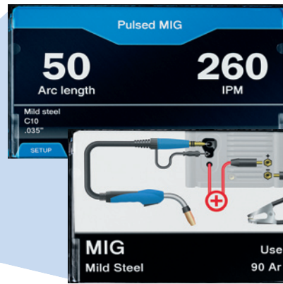
Pulsed MIG setup screen
